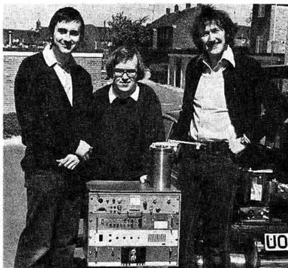
The GB3WS uhf repeater with its main constructors (l to r) Dave Cawley, G3EAO, Dave Holmes, G8FRV, and Andy Betterton, G8FNF. The repeater is operational from Sudbury Upper School at 250ft asl on 434.75MHz in and 433.15MHz out. Output is 10W erp from folded dipoles, and access is by 1,750Hz tone. Time out is after approximately 2min, and when not in use the repeater sends its callsign every 8min.
